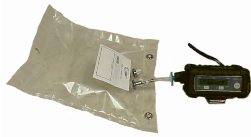
Figure 4-1 Connection of Calibration Gas
