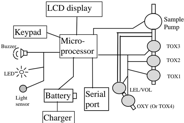
Figure 6.1 Block Diagram of VRAE PGM-7800 Monitor
