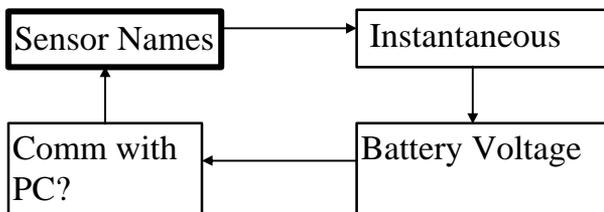
To choose a specific display, press the **[MODE]** key one or more times until the desired display appears.
