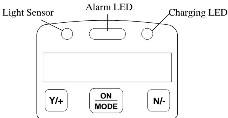
Figure 2.2 Keypad and Display of the VRAE Multi Gas Monitor
